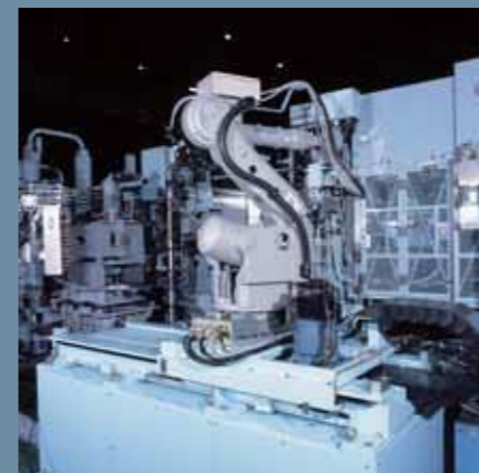
Product Take-out Device Take out robot allows many operations after casting.
